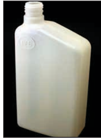
Fig. 3: Blow molded bottle produced from pellet reprocessed with Ceranovus A120 wax
