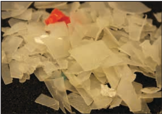
Fig. 1: Natural post-consumer HDPE bottle flake
