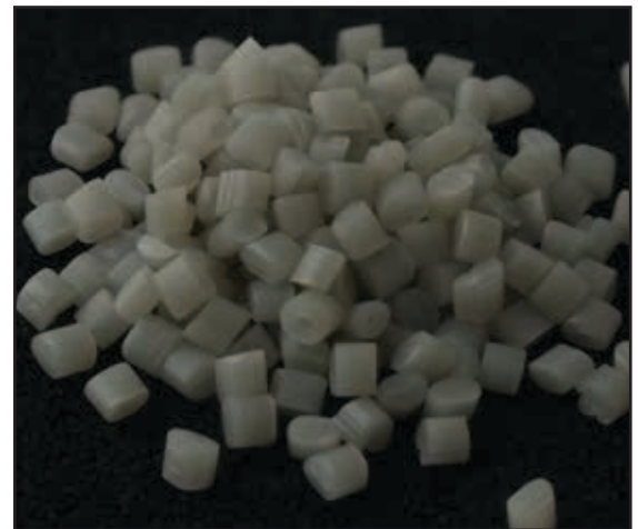
Fig 2: Natural HDPE flake reprocessed to pellet using Ceranovus A120 wax
